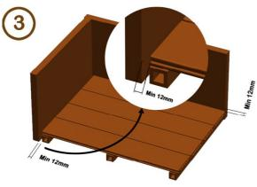
Place the decking on the joist, make sure that the gap between the wall and the decking should be at least 12mm.
