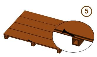
fix the decking and joist with screw from the side groove and in the middle length of decking, Each decking will only need to fix one point.
